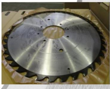
TCT saw-blades of diameters 950mm and 860mm for plate cutting on Sermas plate saws
