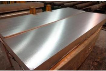
Slab sawing (head + foot cut)
